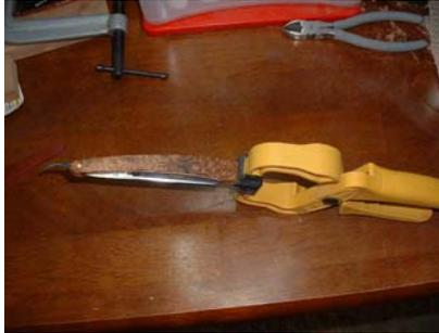
Alright, you're almost done. Take the handle out of the clamp and drill the spacer end. Put a pin through the spacer and follow the same instructions as you did for the pivot end (minus the blade bearings). Now, you will probably have some material that needs trimming around the end, so get out your Dremel or files (whichever you are more comfortable with) and trim it up.
