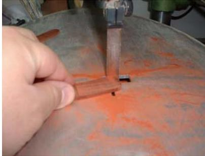
After you have the shape exactly the same for both scales, you are ready to sand the scales. I like to use a C clamp and small scrap piece to hold the scale to the workbench. This will give you more stability and less chance of breaking a scale in half. Start with 220 grit and work out all the saw marks, then move to 320, 400, and 600 respectively.
