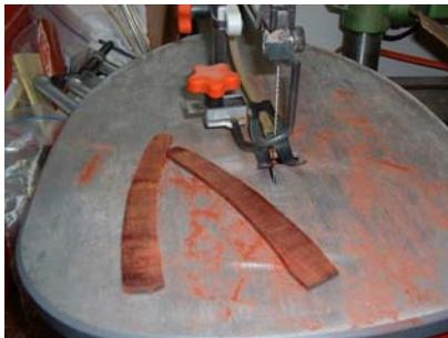
Once you get both scales rough cut, then it is time to sand them to their final shape. I use special sanding strips that fit in the scroll saw, it makes it much faster, and you can use a file or sanding block.
