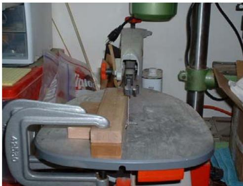
Be sure when you feed the wood through the blade that you do not allow it to chatter up and down. Hold it securely to the bed and fence. Also, your choice of blade should be a single cut 10 TPI blade. The 10 is a little thicker, so it will not “wander” when you feed
